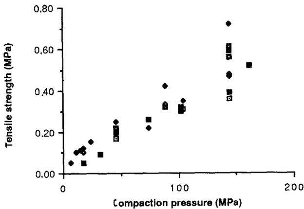
Figure 5 Tensile strength against compaction pressure for different powders. □, TMf; ◆, TMm; ■, TMG; ●, Tg; ▲, D.
