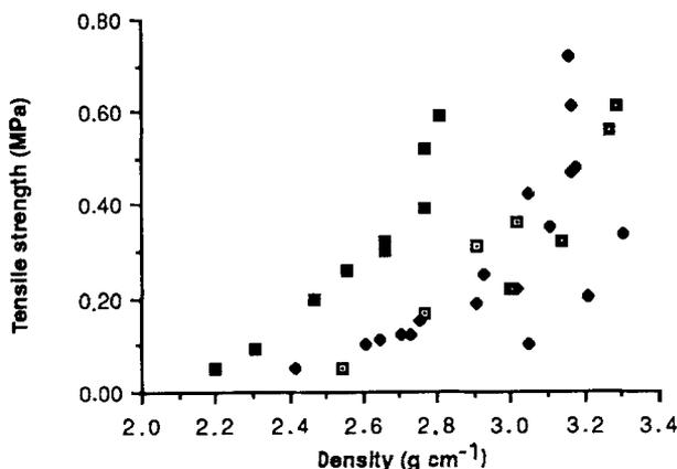
Figure 3 Tensile strength against density for the different powders. □, TMf; ♦, TMm; ■, TMG; ◆, Tg; ■, D.
