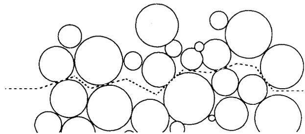
Figure 6 Contacts crossing a plane perpendicular to the compaction axis in 2D.
