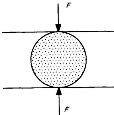
Figure 2 Diametral compression test: the stress state is tensile along the diameter joining the loading points.
