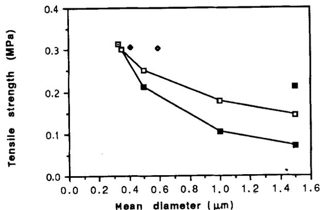
Figure 4 Tensile strength against mean particle size, density  $3.0 \text{ g cm}^{-3}$ . □, TMf; ♦, TMm; ■, TMG; ◆, TM; ■, Equation 3; □, Equation 4.
