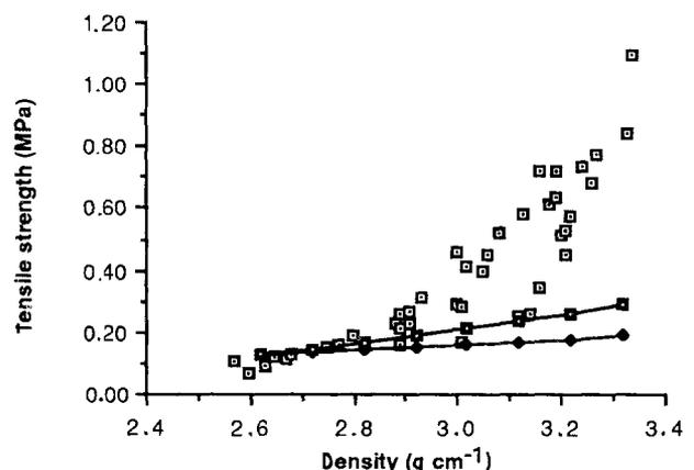
Figure 1 Tensile strength against density, powder TM: comparison between experimental results and theoretical predictions. ♦, Equation 3; ■, Equation 4; □, experiment.
